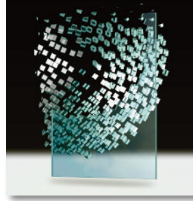
TEMPERED GLASS shatters completely under higher levels of impact energy, and few pieces remain in the frame.
